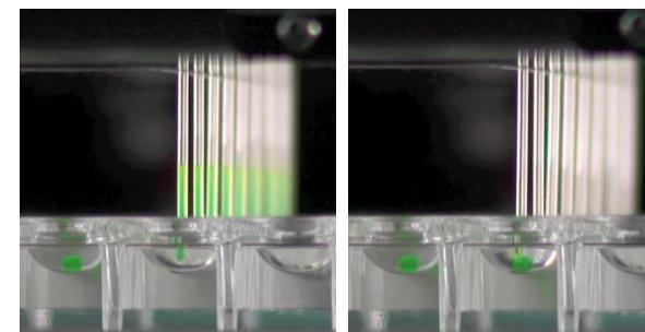
mosquito dispensing a combined drop through oil for microbatch set-up
