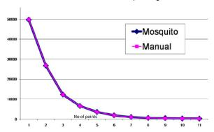
Comparison of mosquito versus manual pipetting for a 1 in 2 11-point serial dilution with 200 nL stamp out into tissue culture treated plate (difficult due to DMSO wicking).
