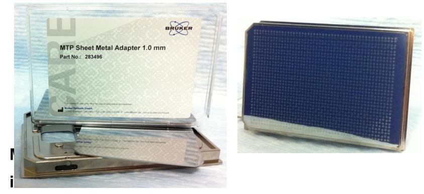
We developed with TTP LabTech a protocol using their Mosquito HTS to enabling spotting of matrix mixed analyte with high spatial resolution in a 1536 format. The system pierces Foil Sealed 384-well plates containing volatile MALDI matrix in 50% acetonitrile, or methanol wash solution. Sample deposition involves: aspirating a 300nL "Sandwich" of 135nL matrix / 30nL analyte / 135nL matrix and depositing them precisely onto the MALDI target.
