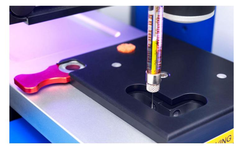
Positioning of the LCP dispense needle relative to the mosquito deck is accurate to +/- 20 µm in the X axis and  $\pm$  5  $\mu$ m in the Y and Z axes.
