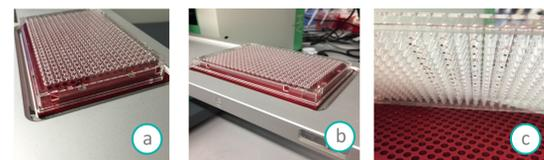
Fig 7. a) and b) magnetic bead plate on mosquito deck, c) beads pulled down using magnetic bead plate.
