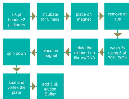
Fig 6. mosquito liquid handler bead clean up workflow.
