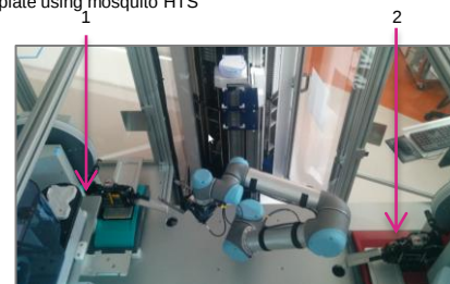
Fig 5. Dart's automated follow-up station with 1) mosquito HTS (diluter) and 2) mosquito X1 (cherry-picker)
