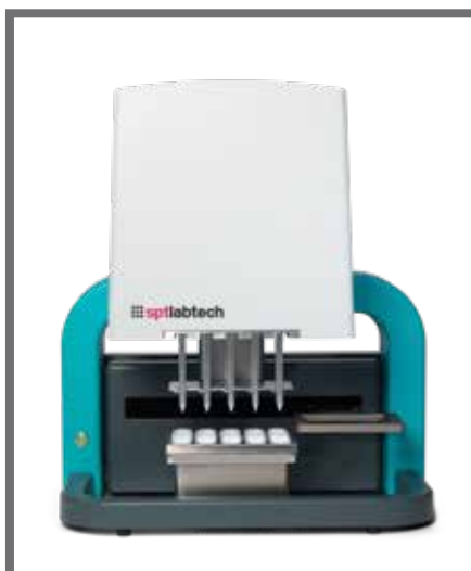
Fig 1. dragonfly ® crystal. The robot has a small footprint and is maintenance-free. To make a screen, the stock solutions are poured into the troughs located on the main stage (up to 10 stock solutions). Syringes are attached to the head of the robot. Once the plate is in place, the formulation protocol is selected before launching the automated making of the screen into the wells of the plate.
