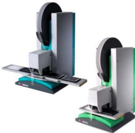
Figure 1. TTP Labtech's mosquito (a) HTS and (b) HV low-volume, automated liquid handlers
