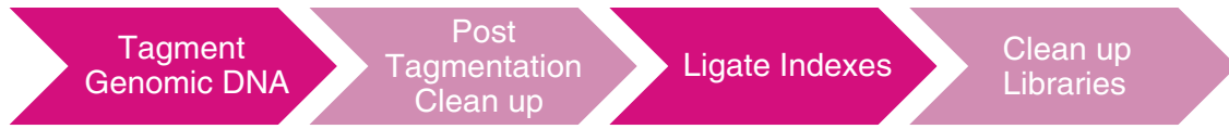
Figure 1. Overview of the steps performed by firefly to automate Illumina DNA PCR-Free Prep.
