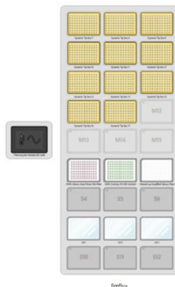
Figure 3. firefly+ starting deck layout for a 96-sample KAPA EvoPlus Boost (or KAPA EvoPlus V2) 3.1-4.3a Fragmentation, Adapter Ligation and Amplification library prep run. Deck layout – Basement: Reservoir R1 – Elution Buffer, R2+R3+R5+R6 – 80% Ethanol, R4 – KAPA HyperPure Beads, Plate Thermal Module - 96 sample Thermo Adapter Block and Input DNA Plate. Lower Deck: L1+L4+L5+L6+L7+L8 L7 - 100 \mu L 96 format ATL tips on ATL 35-125 \mu L Tip Stands, L3 – Waste Plate. Upper Deck: U2 – FragTail ReadyMix Plate, U3 – Ligation ReadyMix Plate, U4 – KAPA UDI Adapter Plate, U5 – Cleaned Up Adapter Ligation Library Plate, U7 – KAPA HyperPure Beads Plate, U8 – Alpaqua Magnum FLX 96 sample Magnetic Block.
