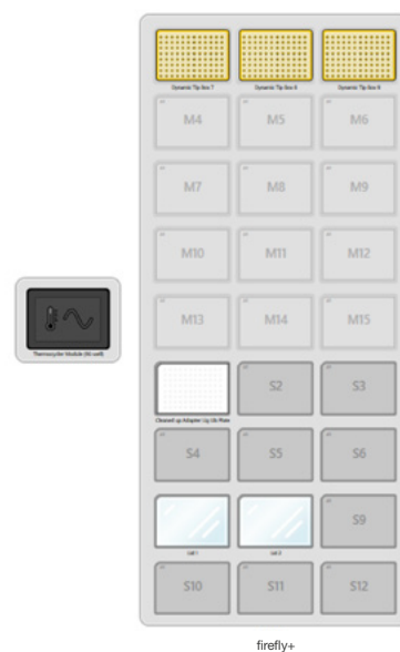
Figure 2. firefly+ starting layout for a 96-sample KAPA EvoPlus Boost PCR-Free 3.1-3.3 Fragmentation and Adapter Ligation library prep run. M1-M3 - 100 µL 96 format ATL tips. S1 – Cleaned up Adapter Ligation Library Plate. S7, S8 – Plate Lids.
