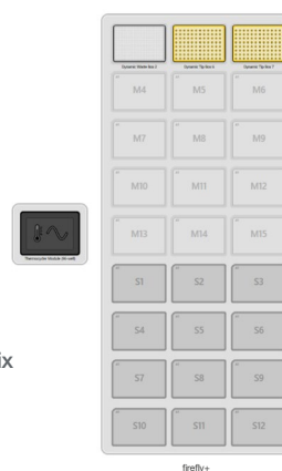
Figure 5. firefly starting deck layout for a 96-sample KAPA EvoPlus V2 Appendix A. Double-sided Size Selection run. Deck layout – Basement: Reservoir R1 – Elution Buffer, R2+R3+R5+R6 – 80% Ethanol, R4 – KAPA HyperPure Beads. Lower Deck: L1+L4+L6+L7+L8 - 100 \mu L 96 format ATL tips on ATL 35-125 \mu L Tip Stands, L5 – Empty Waste tip Box. Upper Deck: U1 – Waste Plate, U2 - Intermediate Plate, U3 – Output Plate, U6 – Input Plate, U8 – Alpaqua Magnum FLX 96 sample Magnetic Block.
