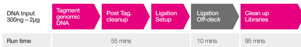
Figure 1. Workflow and firefly® run times for the Illumina DNA PCR-Free Prep kit.
