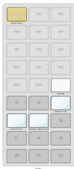
Figure 4 firefly+ starting layout for a 16 sample Target Enrichment run (Part 1). Deck Layout M1 – 100µL 96 format ATL tips, M15 – Waste Plate, S3+S4+S5 – Plate Lids on Plates.
