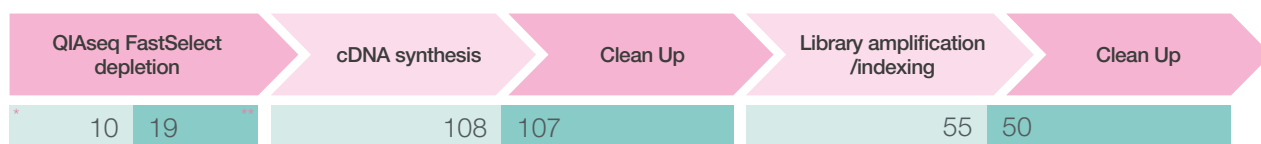
Figure 1. Overview of the steps performed by firefly to automate QIAseq® FastSelect™ RNA Library Kit including HMR RNA removal with run times for firefly and the thermocycler. RNA input: 100 ng.
