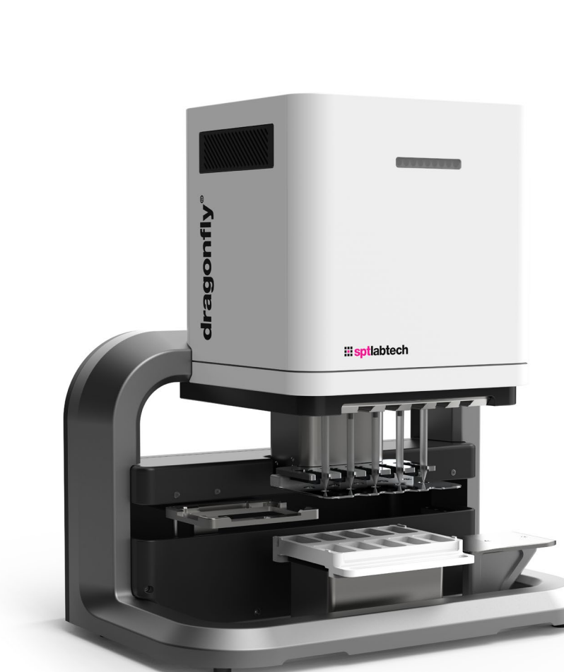
Figure 1. dragonfly discovery is a low-volume, non-contact, positive-displacement dispenser. Each channel is fully independent of the others, yet they can all be operated simultaneously, giving rapid, but highly flexible dispensing. This enables complex combination gradients to be set up in high density (up to 1,536-well) plates, as well as high-speed bulk filling of common reagents.
