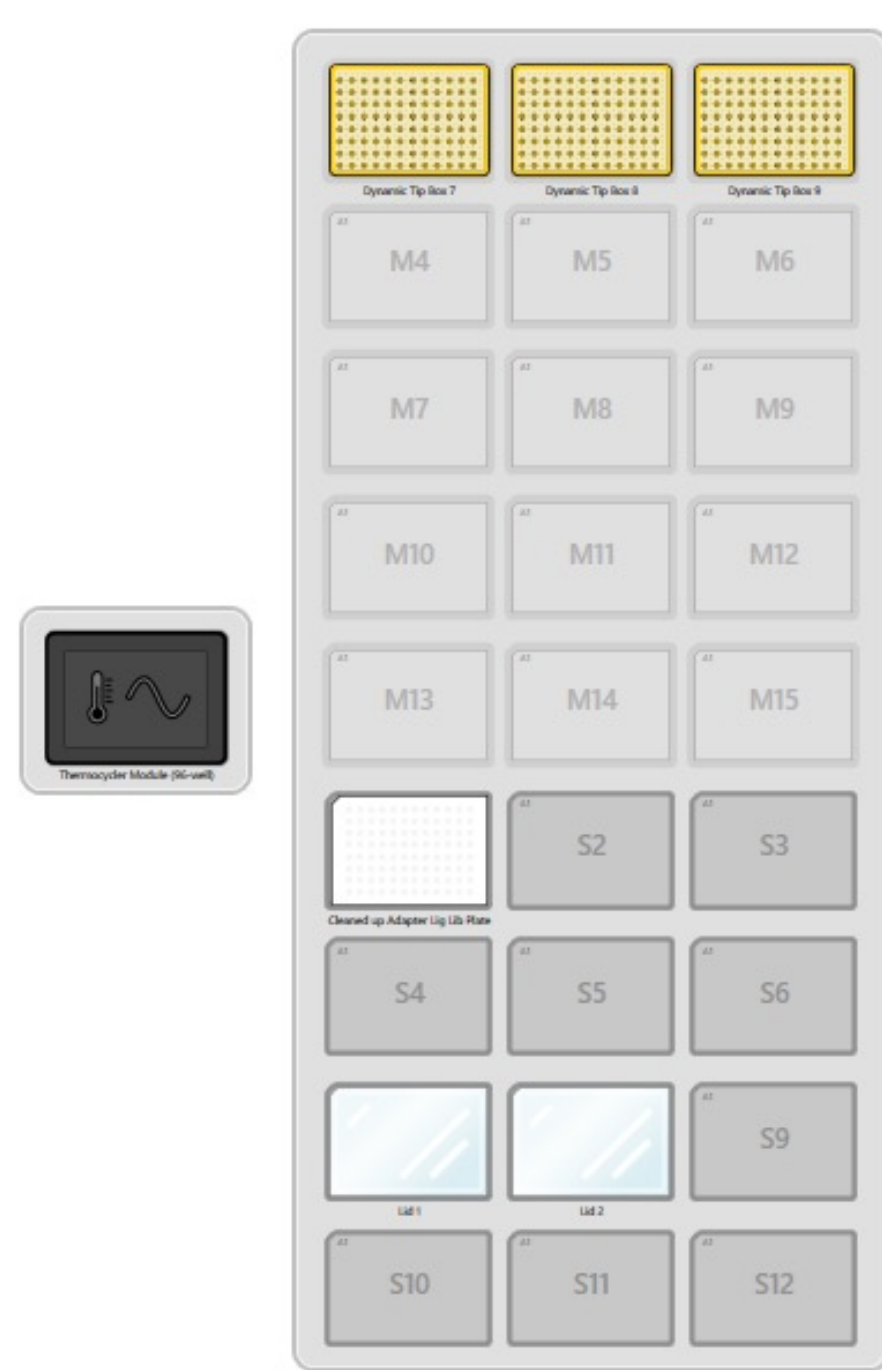
Figure 2. firefly+ starting layout for a 96-sample KAPA EvoPlus Boost (and KAPA EvoPlus V2) 3.1-3.3 Fragmentation and Adapter Ligation library prep run. M1-M3 - 100 µL 96 format ATL tips. S1 – Cleaned up Adapter Ligation Library Plate. S7, S8 – Plate Lids.
